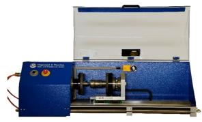
magnetic secure switch during the tests. Only for calibration or service functions the safety door can be deactivated.
