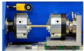
The drive is assembled on the frame of the machine and consists of a servo motor with flanged planetary gear. The mobile carriage with adapted torque sensor is installed at a base plate of steel and directed through a rail guide. The specimen to be tested is clamped between the drive and the mobile carriage using suitable clamping tools (e.g. three-jaw chuck or collet).
